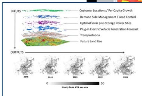
*LoadSEER uses a rich set of geospatial data layers and rule-based land use simulation to determine where new load growth is likely to occur.*
