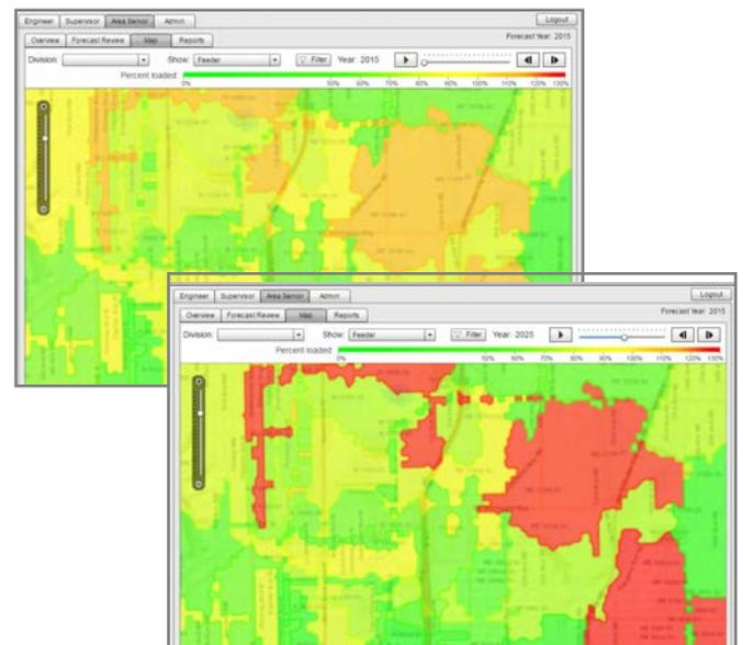
*LoadSEER's distinctively designed to handle multiple scenarios. For instance, the adoption of DERs will affect feeder load shapes and may either exceed feeder capacity from increased load (EV charging station) or may help defer a capacity addition from decreased load (EE/DR/PV). LoadSEER models adoption probabilities for DERs, highlighting which circuits may be at further risk or may benefit from incentivized participation in utility programs.*
