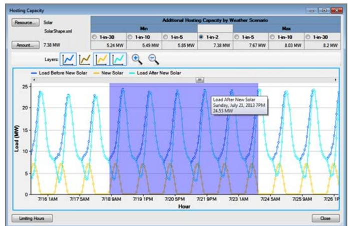
*LoadSEER accommodates DER plans, including Integration Capacity Analysis, subsequent changes in load shapes, and calculating the maximum allowable amount of specific DERs, such as PV.*
